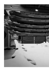
Headliners are given a final quality-control check after being customised to customer requirements.
